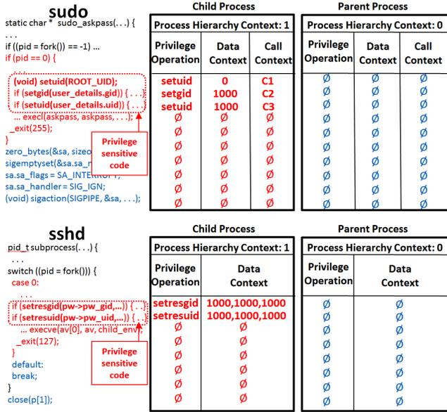
**Figure 1: Automatically extracted multiple process contexts of setuid calls in sudo and sshd. PoLPer prevents any unnecessary setuid calls for the parent process while they are allowed for a child process. PoLPer enforces only required setuid calls based on process context.**
